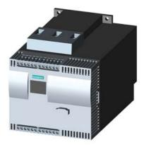
SIRIUS soft starter Values at 400 V, 40 °C standard: 93 A, 45 kW Inside-delta: 161 A, 90 kW 200-460 V AC, 230 V AC Screw terminals !!! Phased-out product !!! Successor is SIRIUS 3RW5, Preferred successor type is >>3RW5527-1HA14<<
