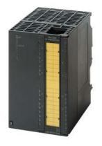
SIMATIC S7, Digital input SM 326, F-DI 24x24 V DC, Fail-safe digital input for SIMATIC S7 F-systems with diagnostic alarm, up to Category 4 (EN 954-1)/ SIL3 (IEC61508)/PLE (ISO13849), 1x 40-pole
