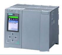
SIMATIC S7-1500, CPU 1517-3 PN/DP, central processing unit with work memory 2 MB for program and 8 MB for data, 1st interface: PROFINET IRT with 2-port switch, 2nd interface: PROFINET RT, 3rd interface: PROFIBUS, 2 ns bit performance, SIMATIC Memory Card required
