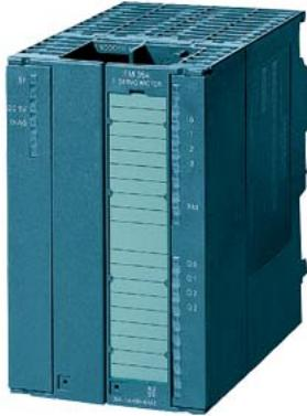
SIMATIC S7-300, FM 354 SUBMODULE FOR POSITIONING WITH SERVOMOTORS, MODULE EXCHANGE W/O PG, PREQUISITE STEP7 V3.1 INCL. CONFIG. PACKAGE ON CD
