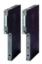
\*\*\*\*\*\*\*\*\*\*\* Replacement part \*\*\*\*\*\*\*\*\* SIMATIC S7-400, CPU 412-2 Central processing unit with: work memory 512 KB, (256 KB code, 256 KB of data), 1st interface MPI/DP 12 Mbit/s, 2nd interface PROFIBUS DP
