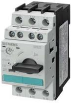
Circuit breaker size S0 for motor protection CLASS 10 A-release 0.11...0.16 A Short-circuit release 2.1 A Screw terminal Standard switching capacity with transverse auxiliary switch 1 NO+1 NC !!! Phased-out product !!! Successor is SIRIUS 3RV2 Preferred successor type is >>3RV2011-0AA15<<
