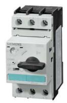
Circuit breaker size S0 for motor protection CLASS 10 A-release 14...20 A Short-circuit release 260 A Screw terminal Standard switching capacity !!! Phased-out product !!! Successor is SIRIUS 3RV2 Preferred successor type is >>3RV2021-4BA10<<
