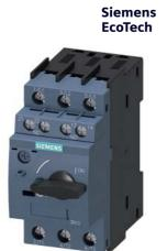
Circuit breaker size S00 for motor protection, CLASS 10 A-release 0.9...1.25 A N-release 16 A screw terminal Standard switching capacity with transverse auxiliary switches 1 NO+1 NC
