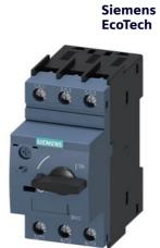
Circuit breaker size S0 for motor protection, CLASS 10 A-release 2.2...3.2 A N release 42 A screw terminal Standard switching capacity
