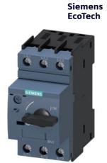
Circuit breaker size S0 for motor protection, CLASS 10 A-release 16...22 A N-release 286 A screw terminal Standard switching capacity
