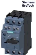
Circuit breaker size S0 for motor protection, CLASS 10 A-release 16...22 A N-release 286 A screw terminal Standard switching capacity with transverse auxiliary switches 1 NO+1 NC
