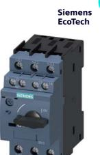
Circuit breaker size S0 for motor protection, CLASS 10 A-release 30...36 A N-release 432 A screw terminal Standard switching capacity with transverse auxiliary switches 1 NO+1 NC
